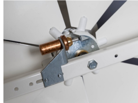
Thermostatic mechanism for blade movement
